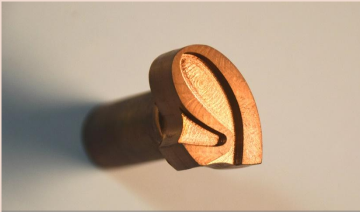
Custom CNC-Milled Copper Logo for Branding Iron
